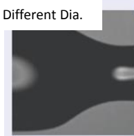
Dissimilar fiber Splicing
